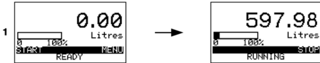
Shows batch quantity, units of measurement & bargraph depicting batch progress.
